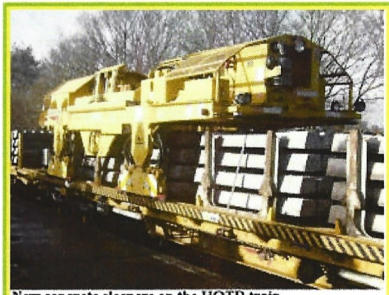
New concrete sleepers on the HOTR train alongside Bow station 16th January
