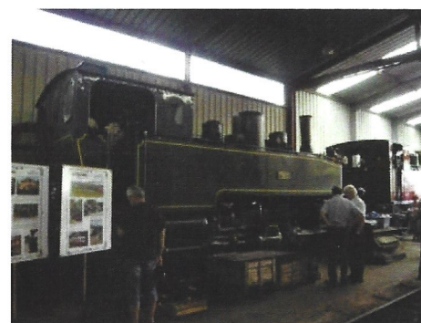
1912 0-4-0+0-4-0 Henschel Mallet inside the shed at Burnhaupt with 1914 No51 0-6-0T in front
