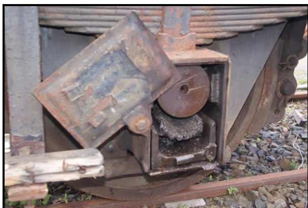
The van's weight being carried on the top face of the axlebox itself, as the bronze and white metal bearing is missing (left). Axle box deformed having been used as a jacking point (right). (J. Kelsey).
