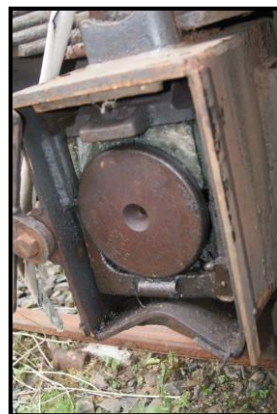
The van's weight being carried on the top face of the axlebox itself, as the bronze and white metal bearing is missing (left). Axle box deformed having been used as a jacking point (right). (J. Kelsey).
