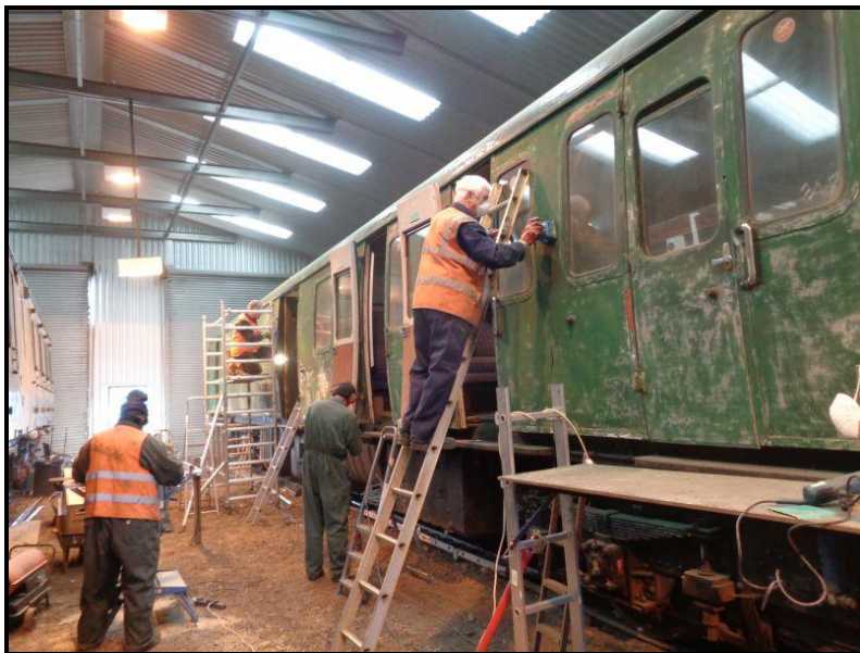
A C&W team sanding down the side of Thumper. This along with any required filling takes the time in the preparation process before painting can begin.
