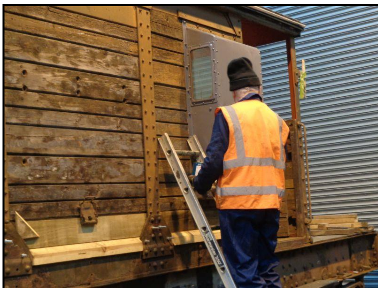
New and rubbed down timbers to the side of the GBV.
