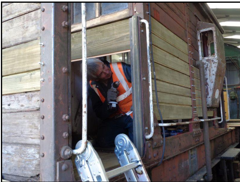
Working on the replacement of timbers to the end and side of the GBV.
