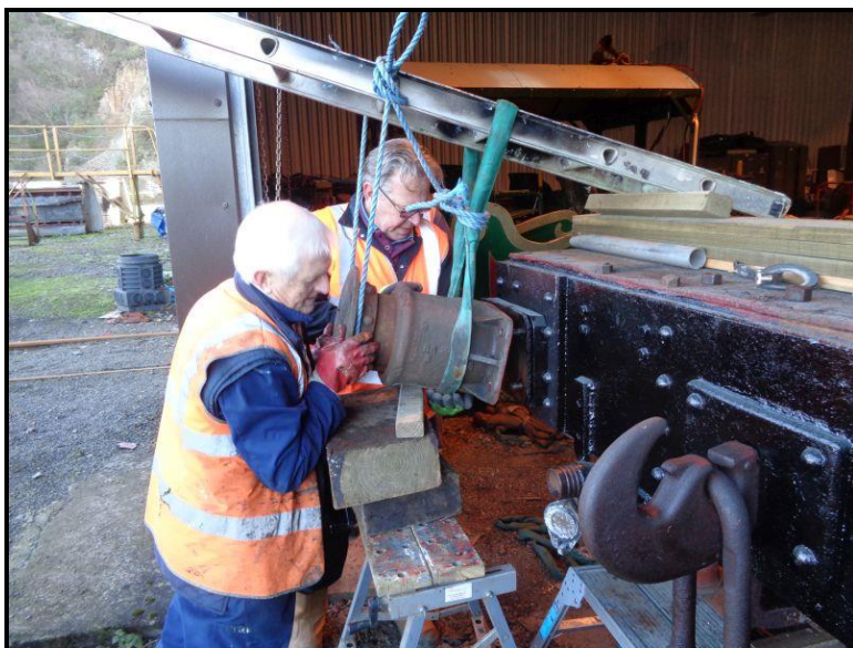
Muscle power employed in refitting one of the buffers.
