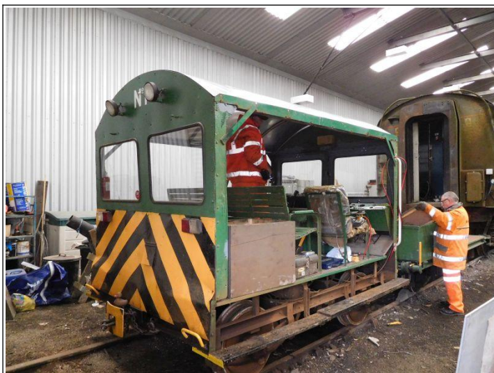
10841 being re-roofed in the Meldon C&W workshop on February 25 th 2016. © Geoff Horner.
