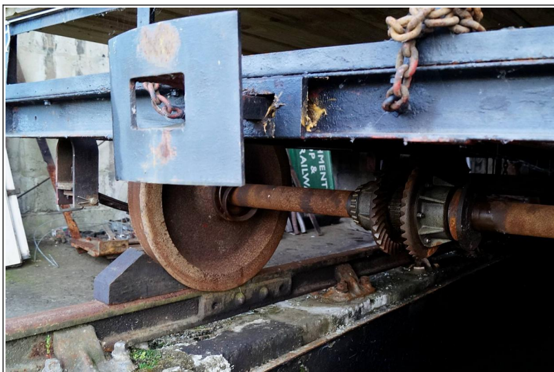
Forward and reverse crownwheels hint at 10842's origins as a powered trolley. June 2015. © Dev-Lak Photography
