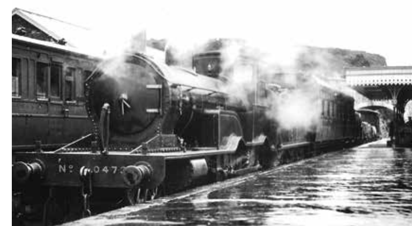
A 460 class express passenger locomotive waits at Torrington Station. Built by Robert Stephenson, entered service as LSWR 473 in June 1884, it was renamed 0473 and transferred to Southern Rail in January 1923 and withdrawn from service in October 1928.
